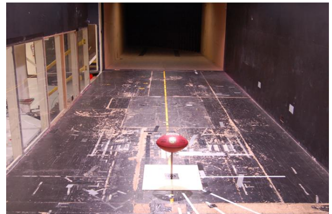
Figure 2. Experimental set up in the test section of RMIT Industrial Wind Tunnel
